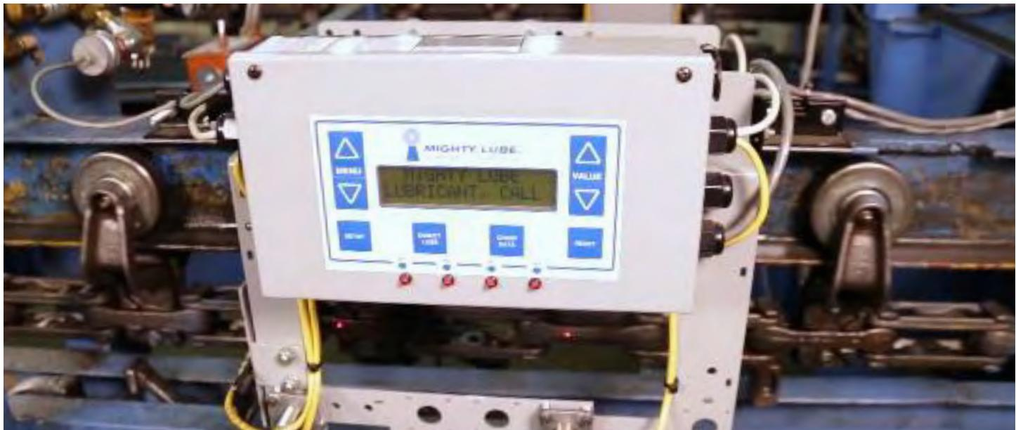
The Conveyor Guardian™ serves as the foundation of an intelligent conveyor maintenance ecosystem, continuously collecting live data on chain wear, vibration, temperature, air pressure, and amp draw to identify optimal lubrication intervals and detect anomalies before they escalate. Its advanced analytics provide a detailed view of conveyor performance through reports and trends such as:
