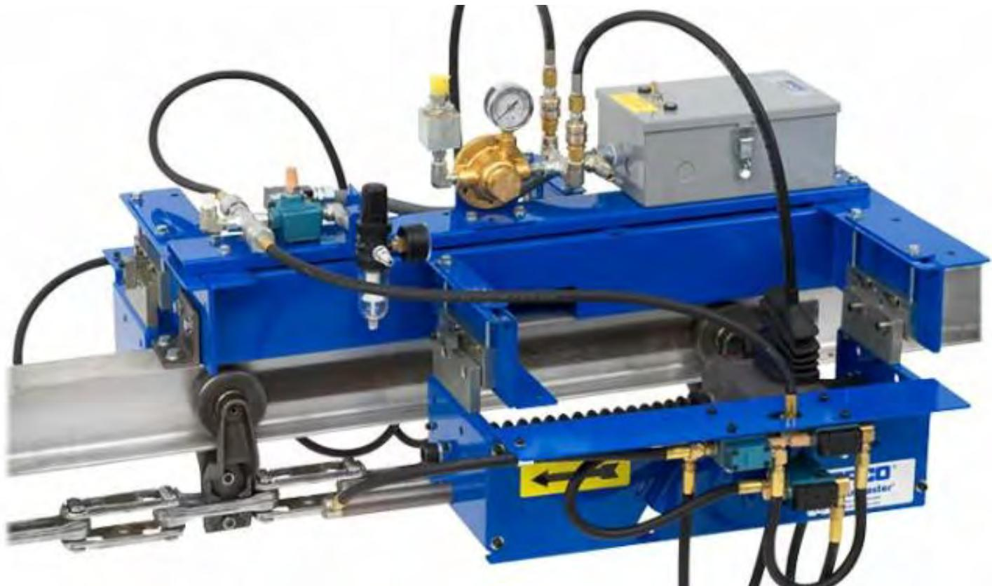
OPCO automatic sealed wheel lubricators are designed for several chain styles, including standard overhead, inverted, roller chain, power-and-free, flat-top, and outboard, inboard, and free-trolley wheel configurations. They lubricate these wheels with precise, metered grease or lubrication while the conveyor is running. This reduces drag, extends component life, and eliminates the labor and waste of manual greasing.
