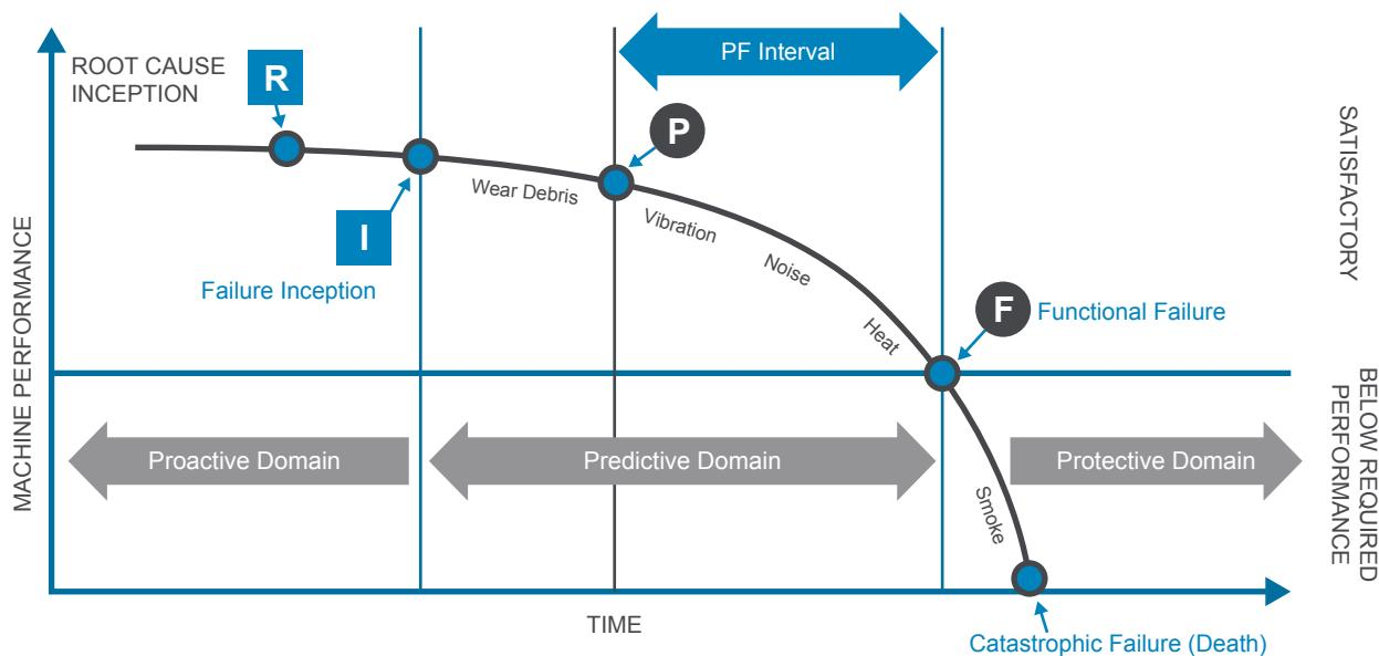
Based on the PF curve, techniques such as vibration and temperature monitoring fall under the predictive domain when specialized technology is used. Any time the P-F curve is extended, there is more time for planning outages, ordering parts, and scheduling labor.
